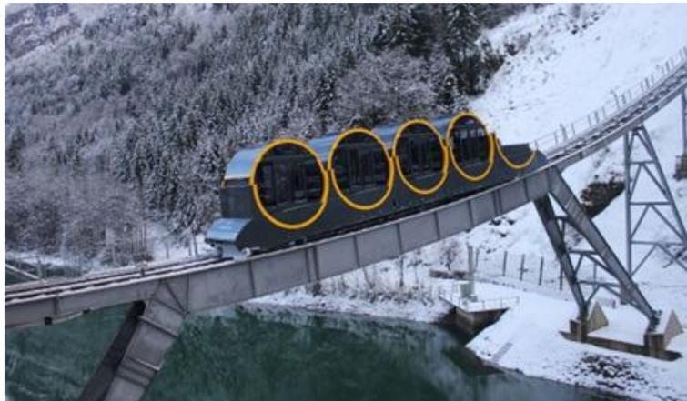
Have you ever seen a funicular? They are a unique cable railway system that works well in steep areas. The Stoosbahn (pictured) in Switzerland is the world's steepest funicular, with a whopping 110% maximum slope or 47.7 degrees. It sure beats having to walk or bike up the hill!
